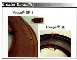
Pyropel is able to maintain dimensional stability and withstand plasma chemistry much longer than competitive products.
