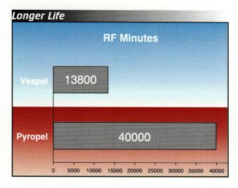
Normally after 15000 RF minutes or less, the fingers and screws are replaced because of severe deterioration caused by the plasma chemistry. Pyropel lasts three times longer.
