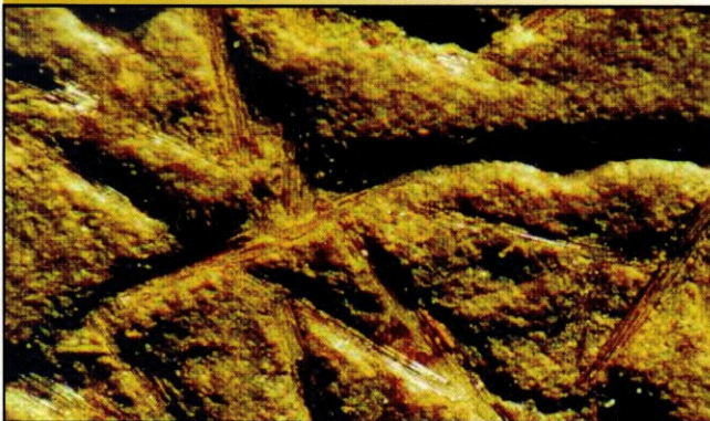
Thermally degraded glass reinforced polyester platen insulation can cause major quality issues if not properly addressed. The above microscopic photograph shows how the polyester binder has been destroyed and only a skeleton remains.
