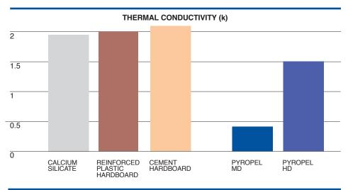
As the graph above shows, Pyropel is 2 to 4 times more effective than other insulation materials typically used in plastics and rubber processing. This superior insulating capability is due to a patented manufacturing process that creates sintered fiber bundles. These bundles give Pyropel its rigidity, compressive strength, and durability. They also trap and hold air which makes Pyropel a highly effective insulator.
