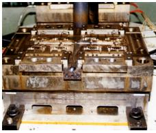
A Pyropel insulation ensures optimum temperature and flow conditions for exotic engineering grade polymers in hot runner injection molding.
