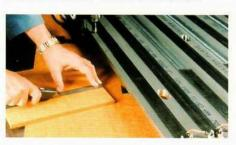
Pyropel is easy to use and requires no special tools. It handles like wood or any free-machining plastic. Pyropel can be drilled, milled, routed, and sawed using standard wood or metalworking tools.
