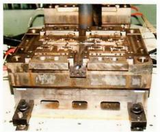
▲Pyropel insulation ensures optimum temperature and flow conditions needed for thermoset compression molding of electrical wiring devices.
